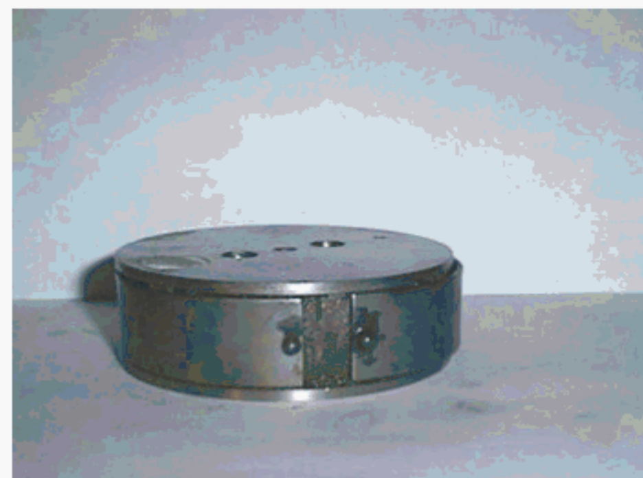
Figure 2 — Typical mould assembly (side view)
