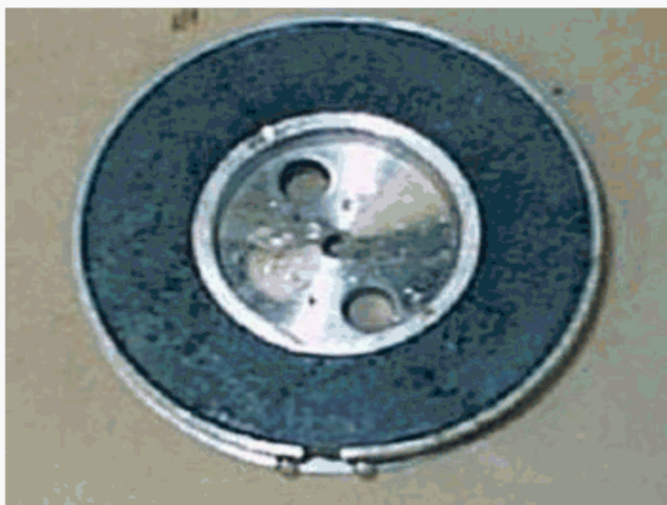
Figure 1 — Typical mould assembly (top view)
