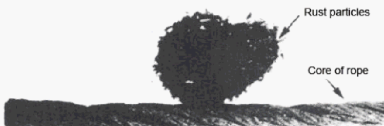
a) Heavy corrosion caused by lack of internal lubrication
