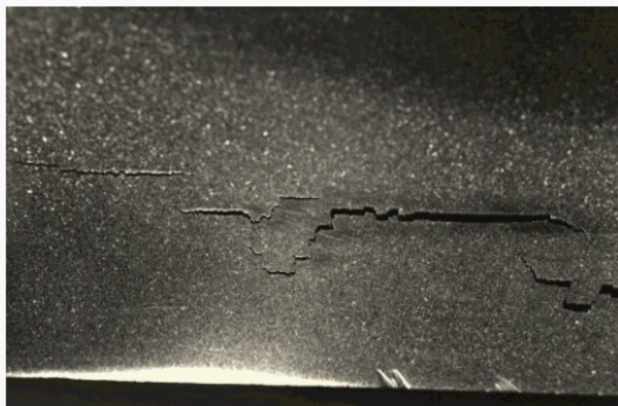
Figure A-2—Hydrogen Blisters near the ID Surface of a Carbon Steel Flange
