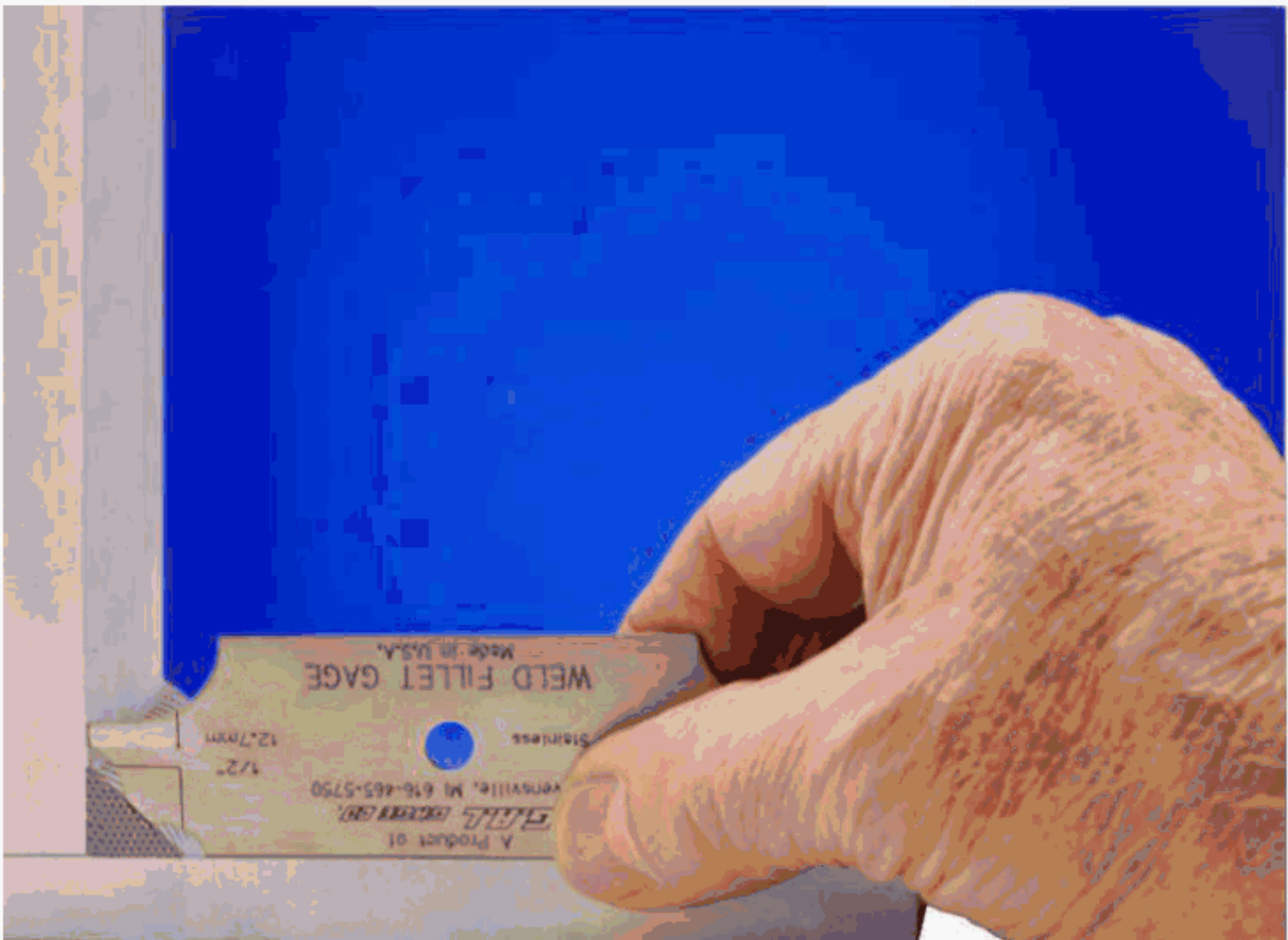
Figure 18—Weld Fillet Gauge
